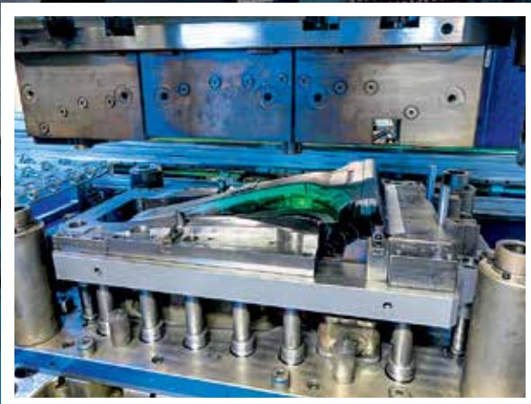
The unformed flat steel slab (above) is turned into a B-pillar in an experimental hot forming tool (left).
