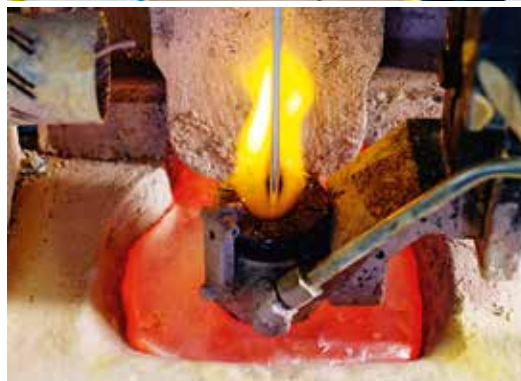
Distribution of roles: Copper-coated hot strips are the source material for the brake lines (above). Coating: A tube is pulled through the liquid aluminum to be coated.
