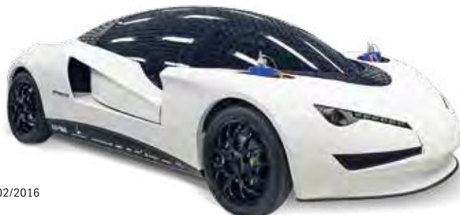
Research vehicle ready for the road: The SpeedE's front end is made out of a steel-CFRP sandwich material.
