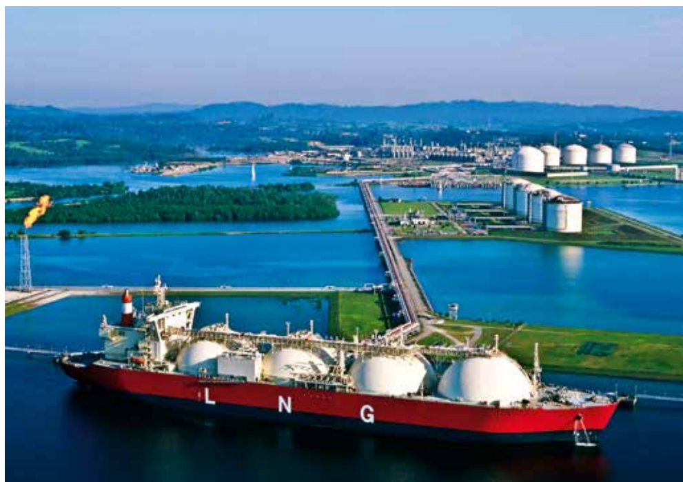
LNG tanker with spherical tanks: Natural gas can be transported by ship in its liquid state.
