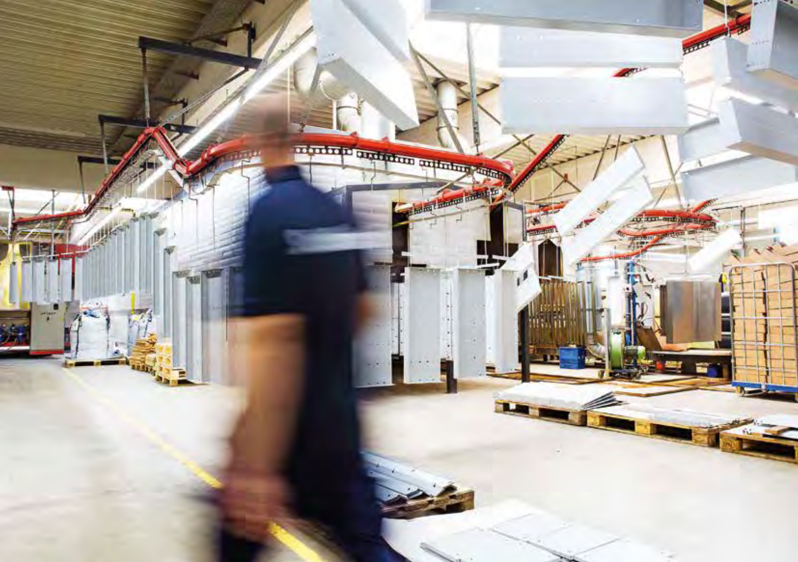
The production carousel keeps turning: The metal frames pass through the coating machine (above), while drawer systems are waiting to be delivered (left).
