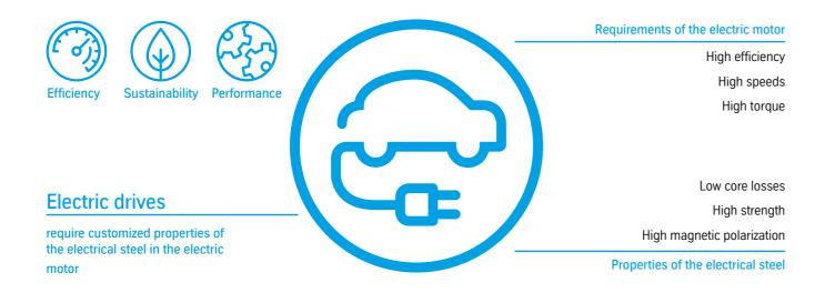
The newly developed top grade for electric mobility 025-125Y420 – which is particularly thin at just 0.25 millimeters – features minimum core losses and a high mechanical strength  $(R_{20,2})$  of at least 420 MPa thanks to an optimized alloy concept. It has proven possible to reduce core losses from max. 14 W/kg (027-140Y420) to max. 12.5 W/kg (at 400 Hz and 1 T) compared
