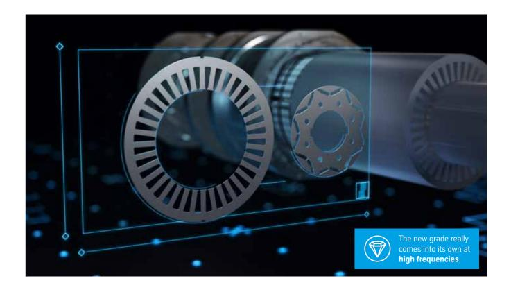
High-speed drive motors in modern electric vehicles not only require excellent magnetic properties, they also place exacting demands on the mechanical properties of the electrical steel primarily on the strength of the material. The high strength of 420 MPa offers the necessary reserves of strength even for highperformance drives, with the possibility of positively influencing the motor design, for example in terms of compactness.
